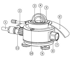
pyranometer (3), glass domes (5), black detector surface (4), sun screen (6), desiccant indicator (7), levelling feet (9), bubble level (10), connector (11).
